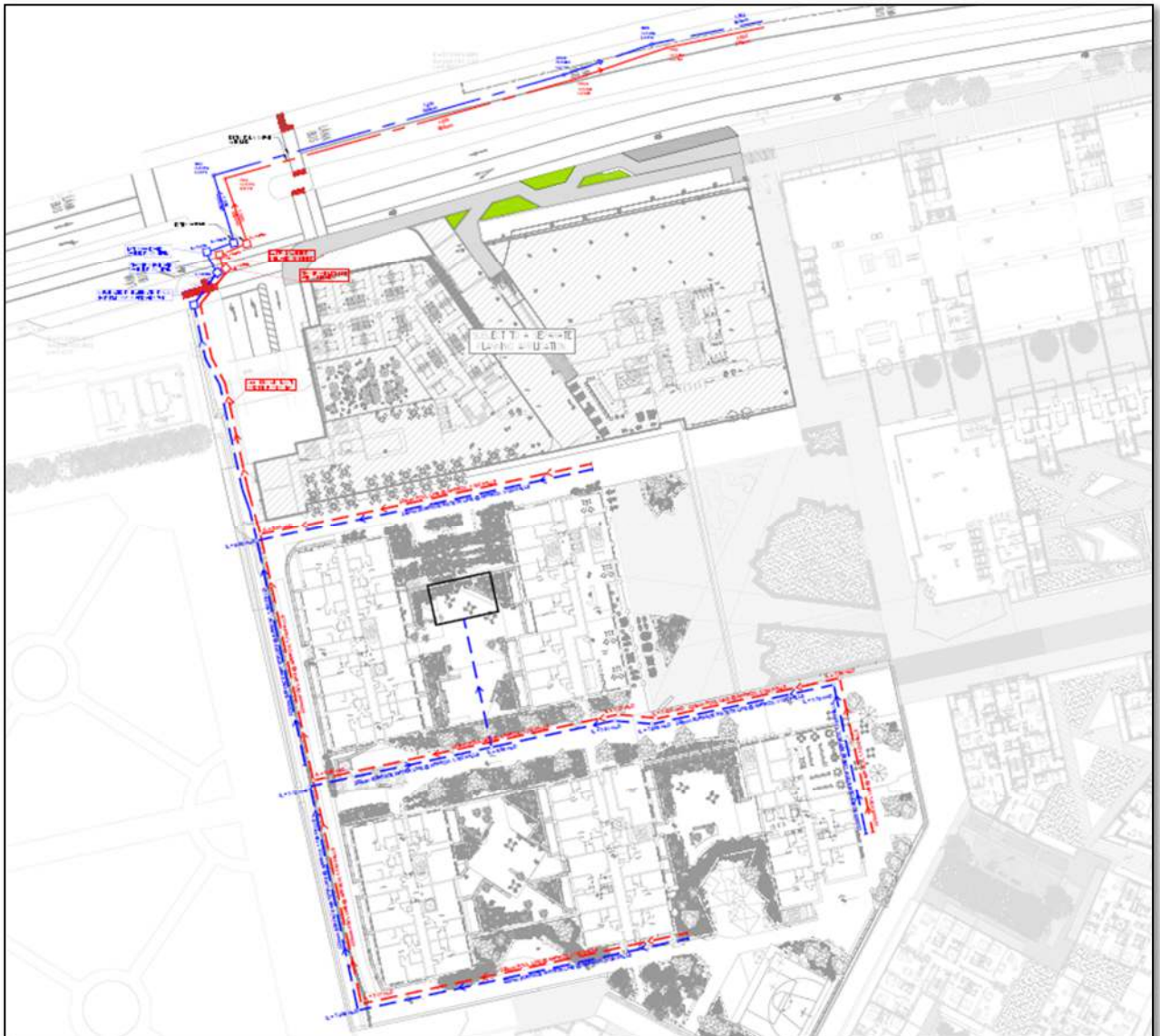
Figure 12.4.1.5 Excerpt from Drawing no. HSQ-CSC-CC-BI-DR-C-0102 showing the proposed drainage infrastructure and routing plan.
