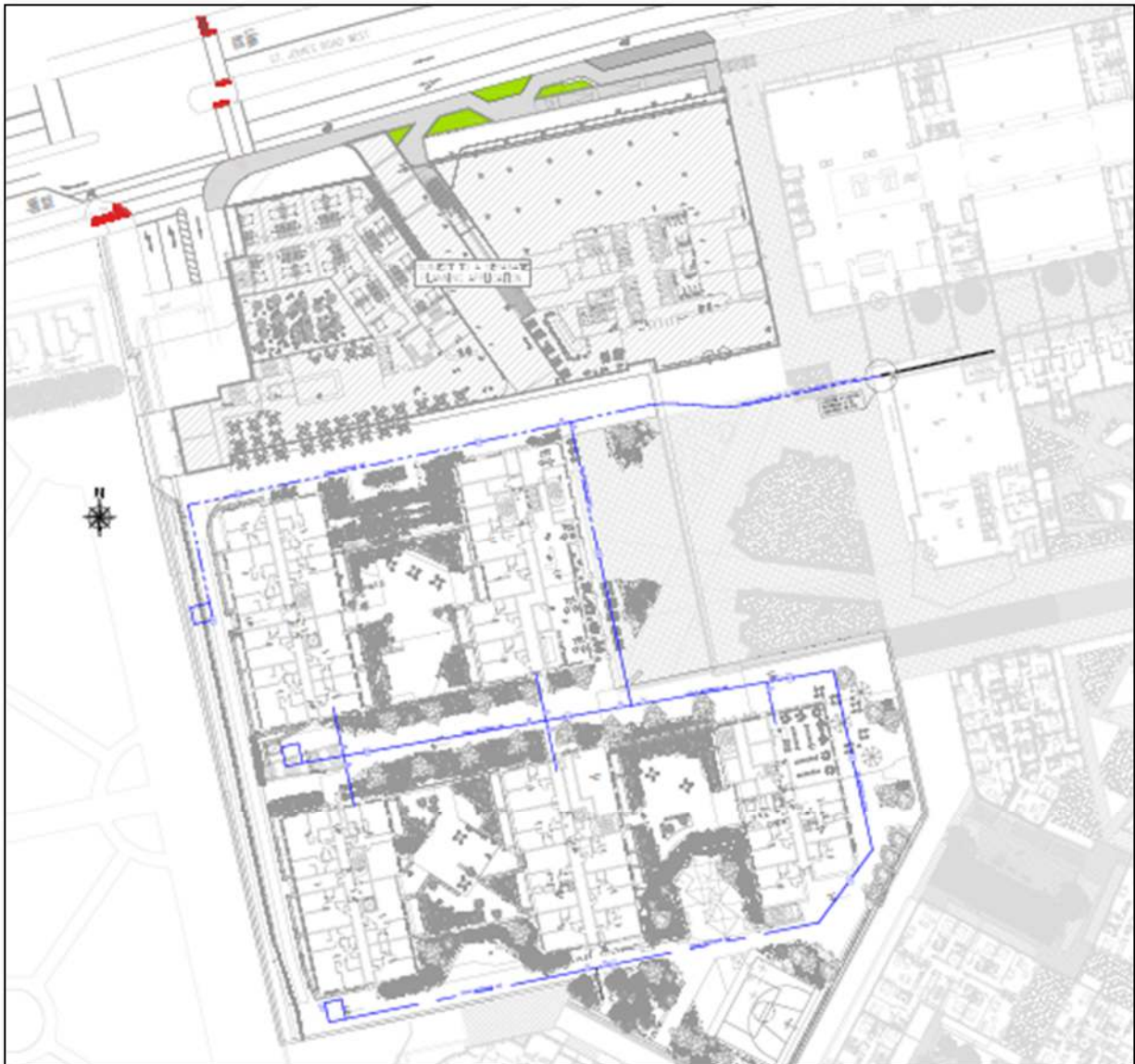
Figure 12.4.1.5 Excerpt from Drawing no. HSQ-CSC-CC-BI-DR-C-0103 showing the proposed potable water infrastructure and routing plan.
